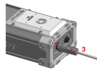
• Push your adapter connector (3) into the Power Pack's connector (4)
