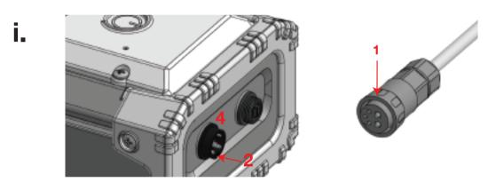
Align the 2 tabs on your motor connector (1) with the two notches on the battery output (2).
